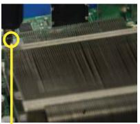
Using a screwdriver to remove Screw#1
